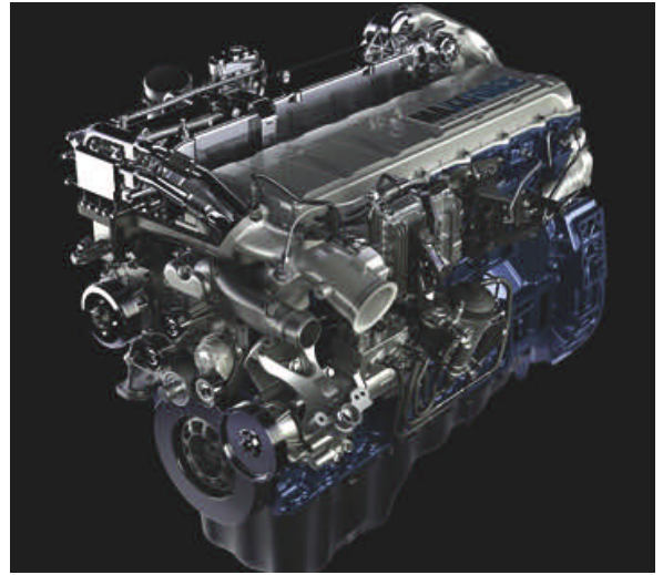
The MaxxForce 11/13 International engines from Navistar for 2010 on-road application comply with 2010 emissions regulations with Advanced EGR, a high-pressure common rail system to provide electronic control and programmability capable of multiple injections per combustion event. Other key elements include proprietary combustion bowl design, advanced air management with dual turbochargers, and electronic calibration strategies to optimize fuel economy and performance.
